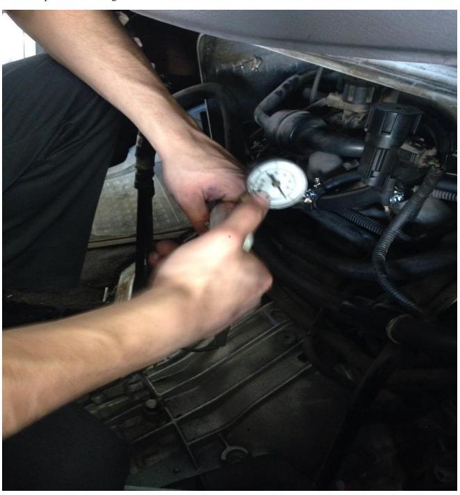
FTPS – STAYED READING -3.75V. A NEGATIVE NUMBER MEANS A VACUUM IS PRESENT COMPARED TO A POSTIVE NUMBER WHICH MEANS PRESSURE.
