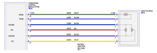
Since both PIDs show high voltage on the signal wires, common components were looked at. Since both signals were showing almost 5 V, power wire was assumed in good condition at this time. Both sensors also shared a common signal return wire. This wire was tested for continuity. PCM connector C175E was removed for this testing. The following measurement was taken: C175E Pin 28 to C1368 Pin 4 resistance read OPEN.
