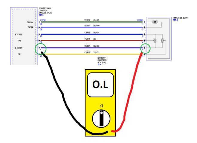
Upon this finding, with an open signal return circuit (RE427 BU-OG), signal wires would read full voltage drop and therefore give us the PID readings from earlier. Recommend repair of Circuit RE427 BU-OG and retest.
